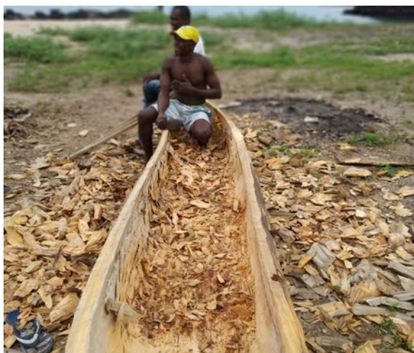
Construction of a cayuco from a kapok tree, San Antonio de Palé, Annobón Island ©FAO/Ricardo Domínguez
